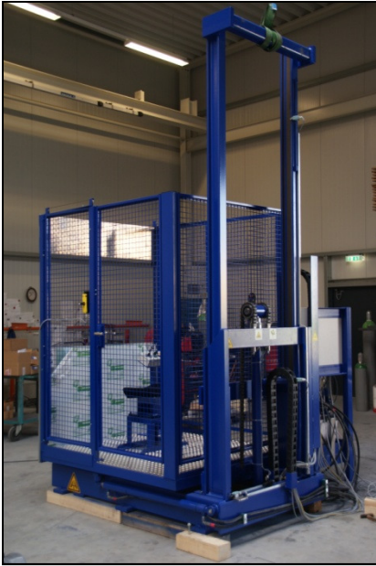
Lifting platform with floor mounting and adjustable recess for spiral machining
