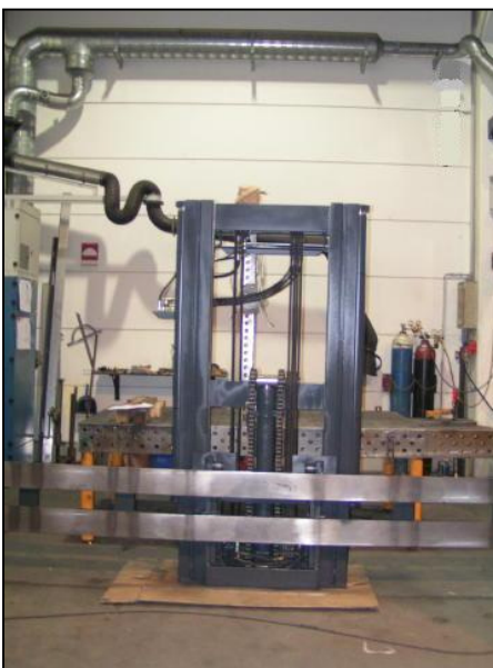
Lifting mast with a lifting fork propensity for side loader
